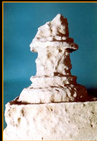
Parts of the original balustrade at Castle Coole, removed during restoration, show obvious loss of architectural detail associated with the combined action of chemical dissolution and physical disruption by salt crystallisation.
