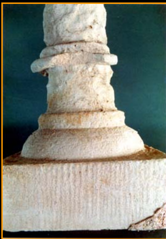
Parts of the original balustrade at Castle Coole, removed during restoration, show obvious loss of architectural detail associated with the combined action of chemical dissolution and physical disruption by salt crystallisation.
