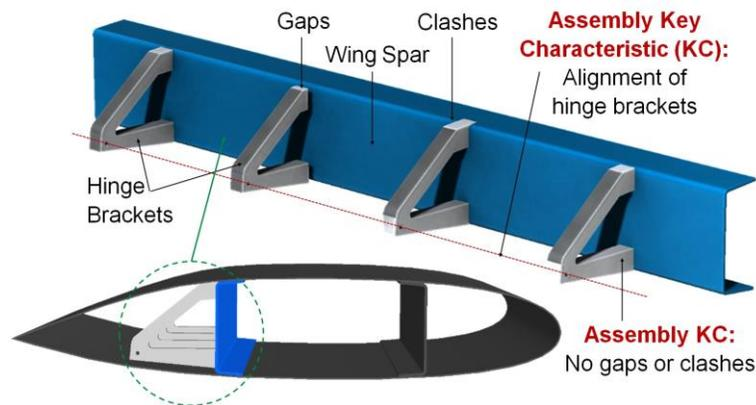
Fig. 1 variation propagation effects on assembly key characteristics
