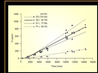
Fig 5. Diffusion rates of chloride through samples of Dumfries Sandstone (D1, D2, D3) and Portland Limestone (P1)
