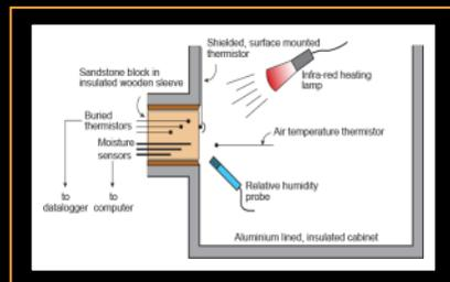
Fig 3. Traditional salt weathering investigations with surface wetting and drying
