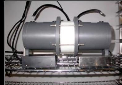
Fig 4. Experimental set-up of diffusion cells
