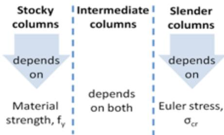
Figure 2: Resistance of columns depends on different factors
