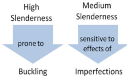
Figure 1 Behaviour of columns is determined by their slenderness
