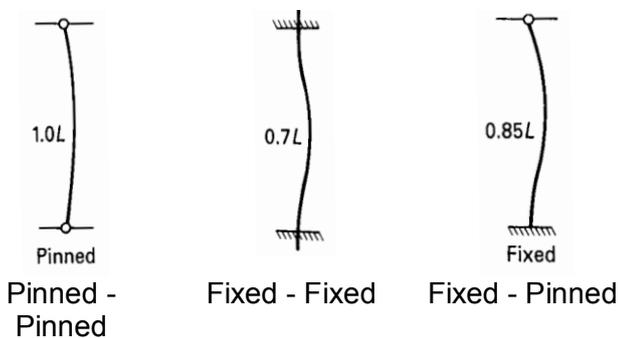
Figure 3: Effective Lengths for three types of end conditions
