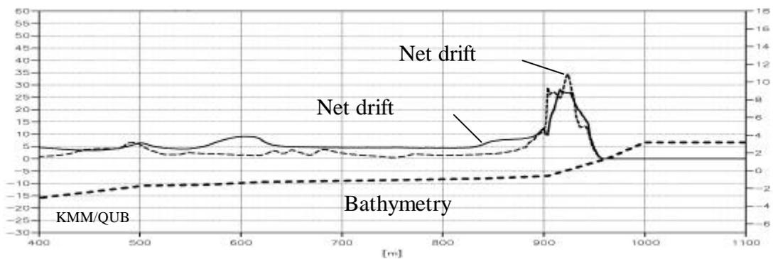
**Figure 8d: net potential sediment transport induced by natural waves and waves due to fast ferries**
