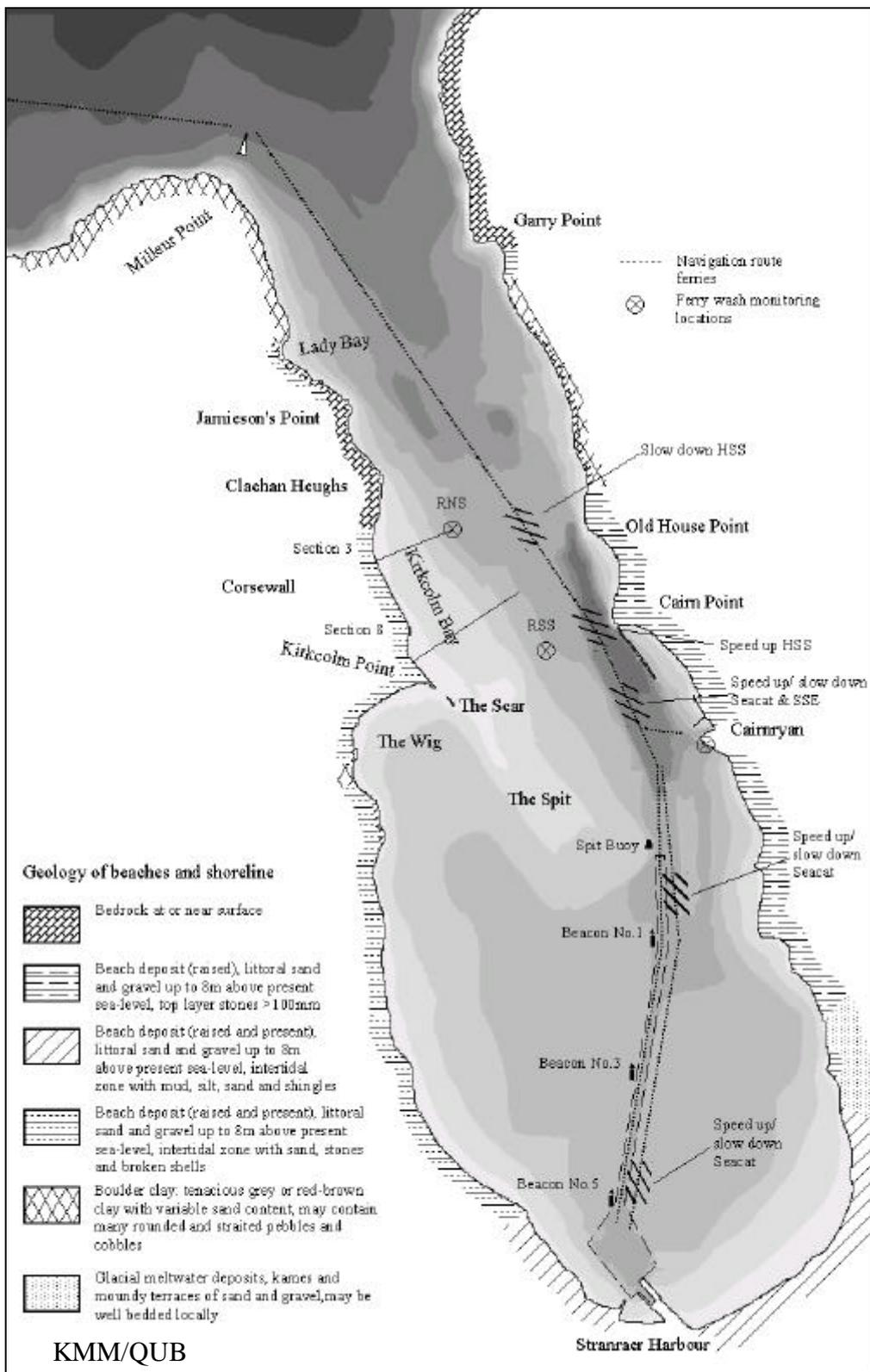
**Figure 1: Loch Ryan - Bathymetry, navigation routes and geological formations along the shoreline**
