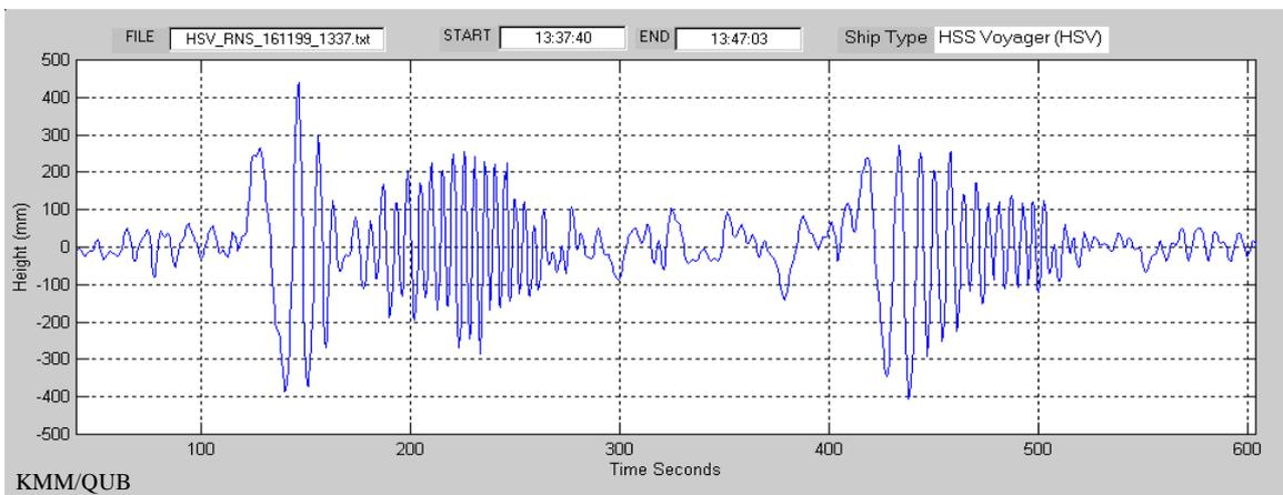
**Figure 7: Fast Ferry wash @ RNS Stena Voyager followed by P&O Jetliner**
