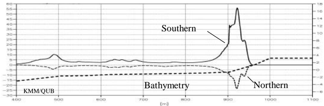
**Figure 8c: potential sediment transport induced by waves due to fast ferries**
