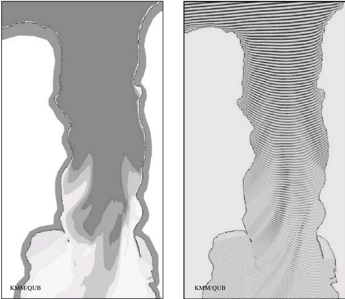
**Figure 6: The natural wave heights and the refraction of waves penetrating into Loch Ryan from the Irish Sea**
