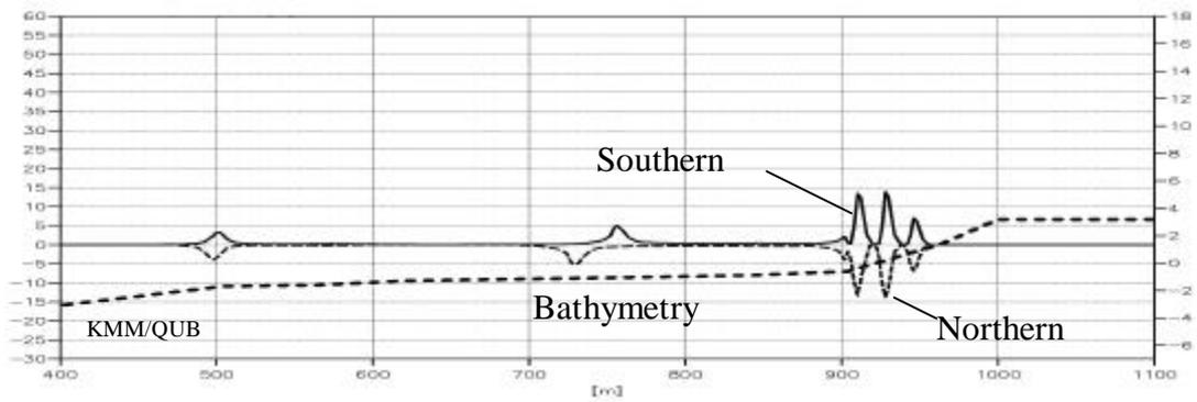
**Figure 8b: potential sediment transport induced by waves due to conv. ferries**
