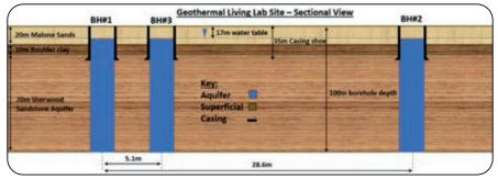
Figure 7 - QUB Geothermal Living Lab
