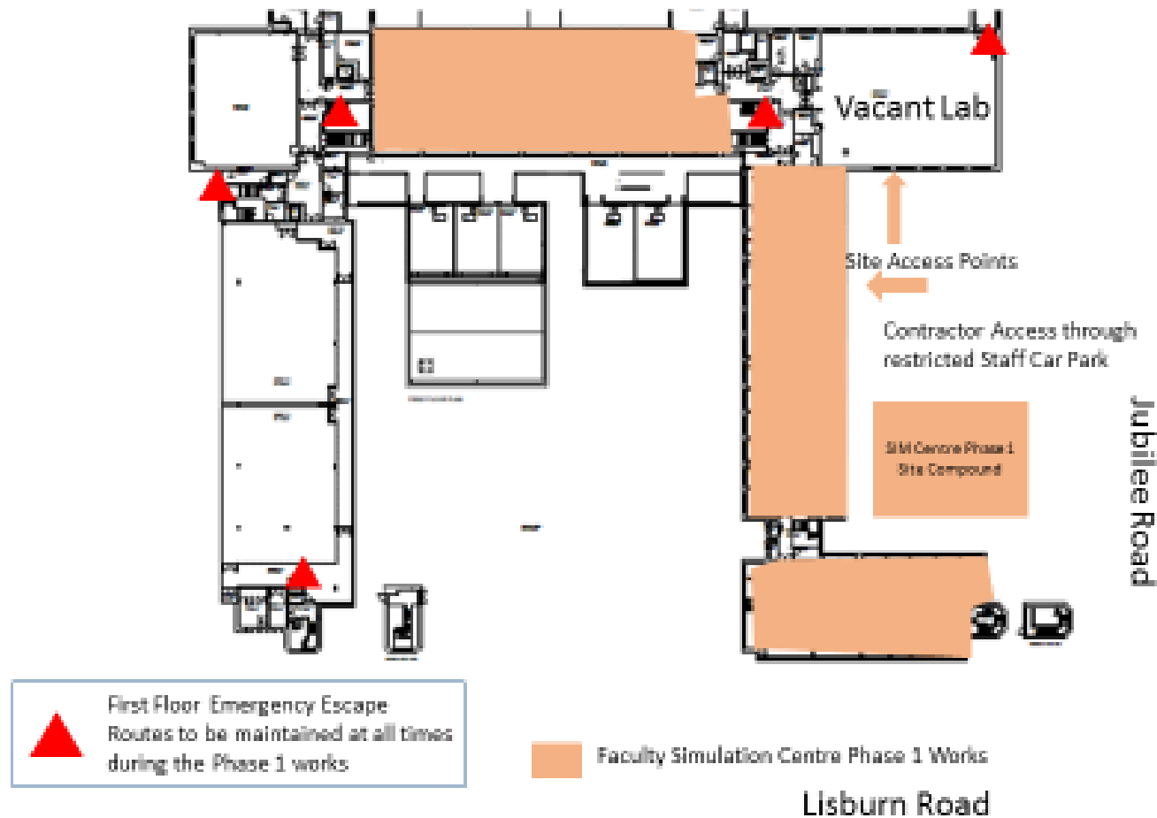
Site Plan: Indicating extent of Phase 1 Works
