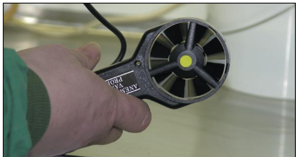
Figure 17 Using a vane anemometer
