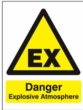
Figure 3: Example of an explosive atmosphere sign.
