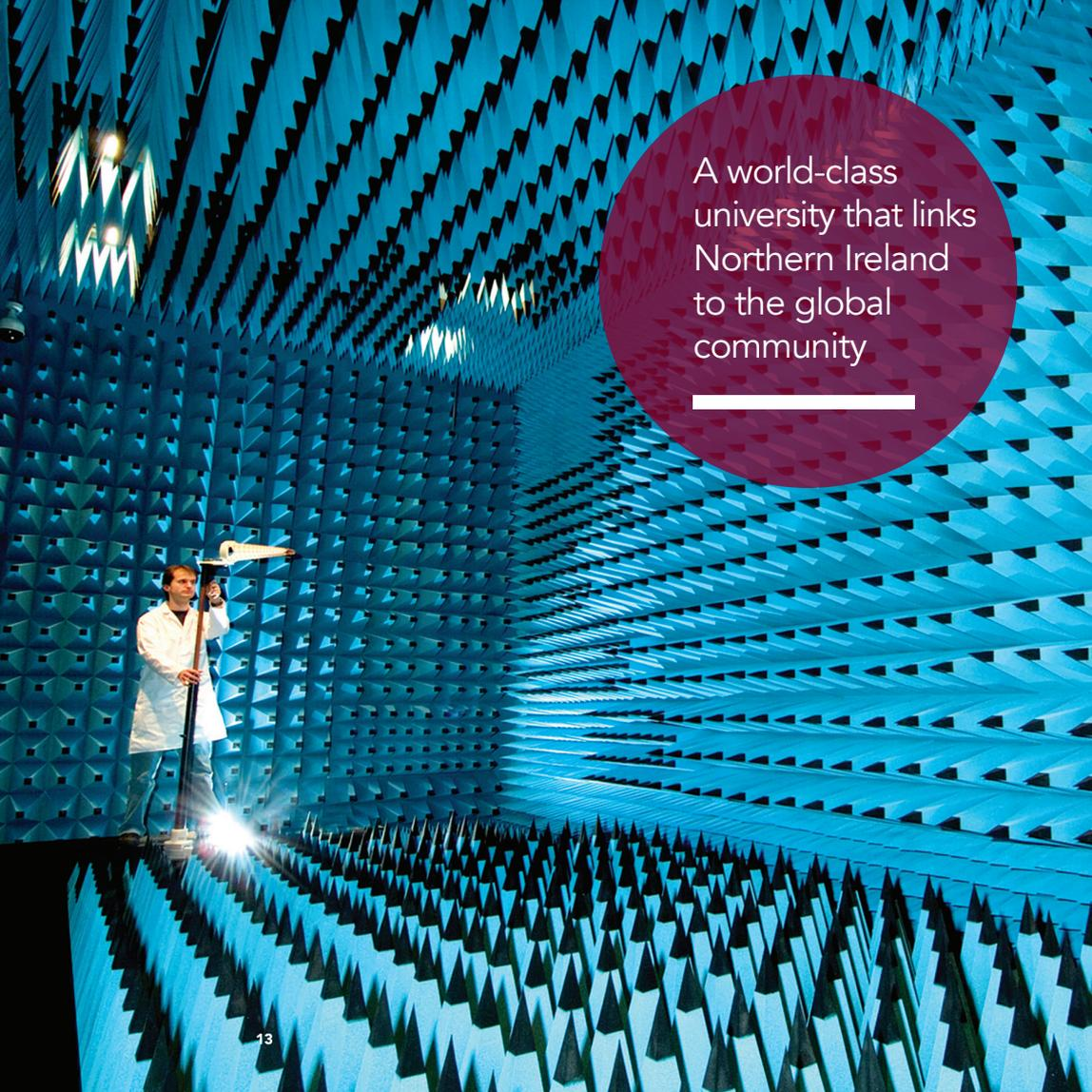
A photograph of a person in a white lab coat standing in an anechoic chamber. The chamber is filled with blue, pyramid-shaped electromagnetic absorbers. The person is holding a large, white, horn-shaped antenna. The lighting is dramatic, with a bright light source on the floor creating a strong reflection. The perspective is looking down a long, narrow corridor formed by the absorbers.
