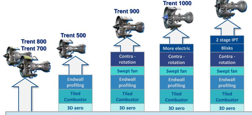
Three shaft architecture, SPF/DB fan, Phase 5 combustor, FADEC
