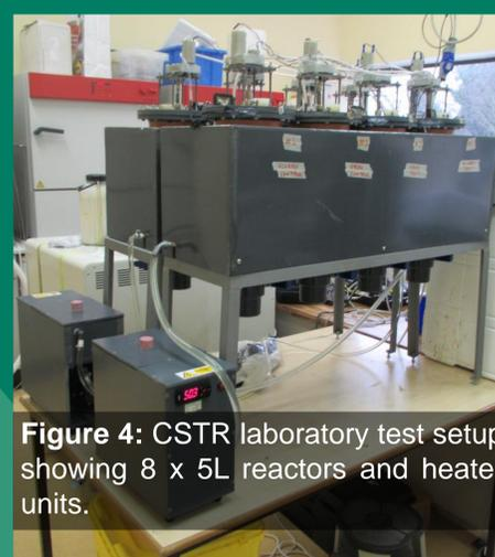
Figure 4: CSTR laboratory test setup showing 8 x 5L reactors and heater units.
