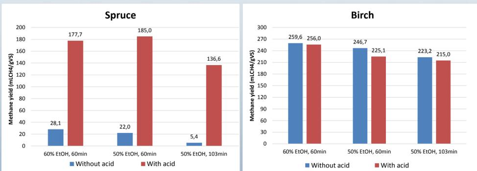
Figure 2. Effect of different pretreatment conditions on the methane yield from spruce and birch chips without the addition of enzymes.
