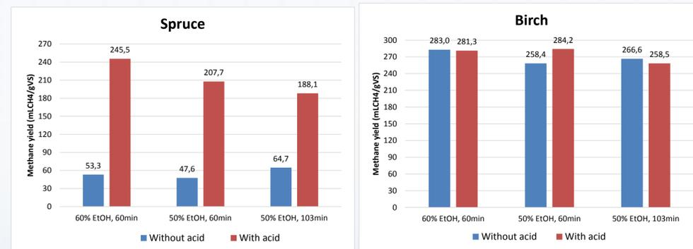
Figure 3. Effect of different pretreatment conditions on the methane yield from spruce and birch chips with the addition of enzymes.
