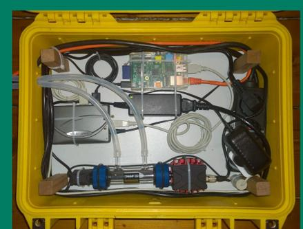
Figure 4 – Inside enclosure showing electronics and MEMS spectrometer.
