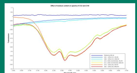
Figure 2 –  $\text{CO}_2$  and  $\text{CH}_4$  spectra for dry gas, and nearly saturated gas.
