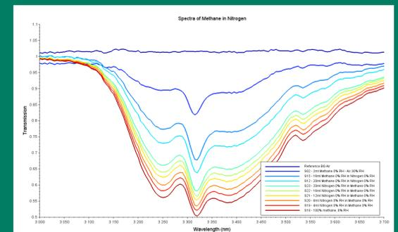
Figure 1 – Methane absorption profile for differing concentrations
