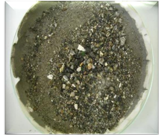
Bottom ash from MSW plant
