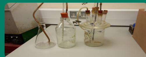
Fig. 1. Lab-scale 1L reactor
