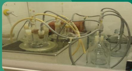
Fig. 2. Lab-scale 1L reactors in water bath
