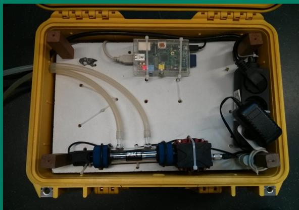
Figure 1 – Gas sensor and raspberry pi mounted in pelican case
