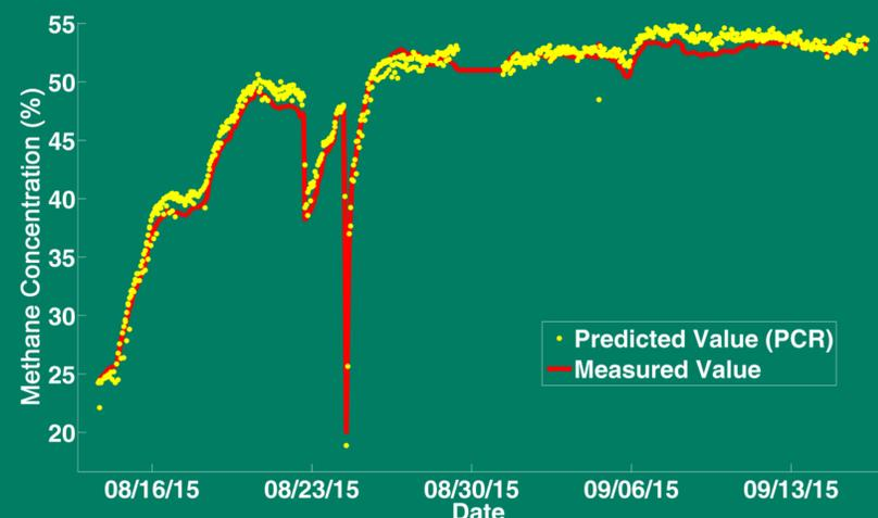
Figure 2 – Predicted methane concentrations plotted against measured test data.
