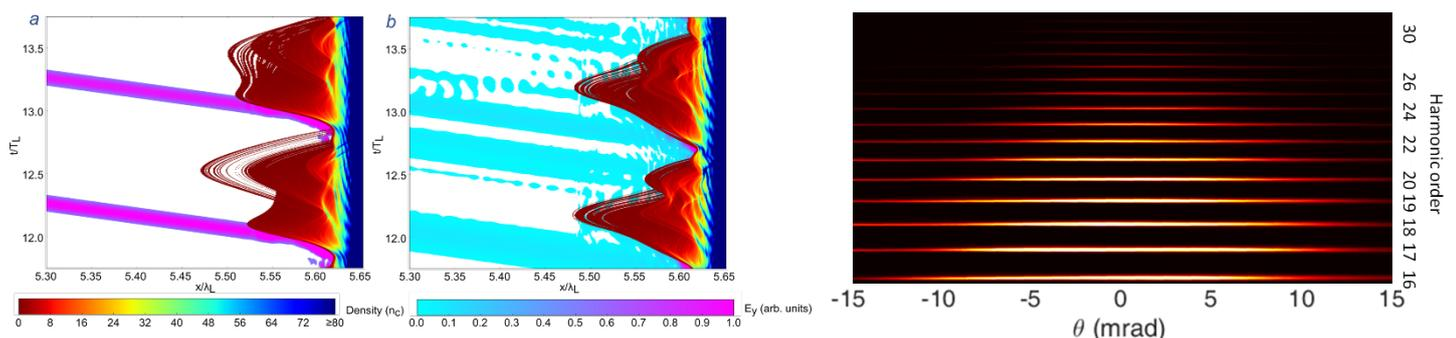
Figure 1 – Left: Simulations of bright, coherent, ultrashort pulses of light when a synthesised multi-harmonic driving pulse is (a) optimised and (b) deoptimized. Right: Experimentally measured beams of high frequency harmonic radiation (as a point of reference, 20<sup>th</sup> harmonic is 40nm wavelength) generated from laser irradiation of a solid density plasma surface at the JET140 laser facility in Jena, Germany.
