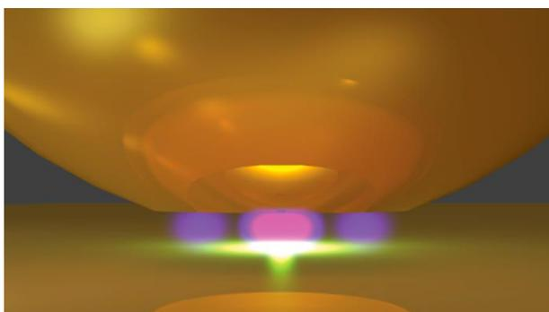
Fig.1 Schematic of a nanoparticle-on-mirror plasmonic nanocavity[1]
