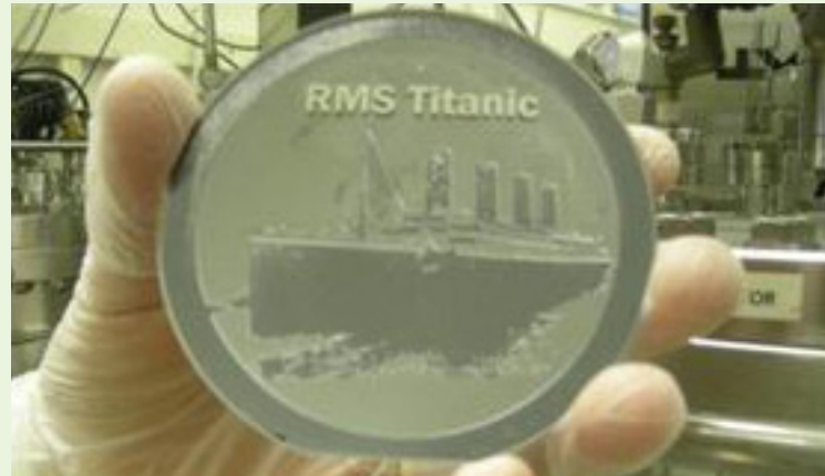
Commemorative image of the Titanic etched into silicon and bonded to a glass substrate
