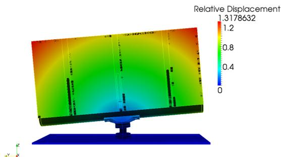
Oscillating Wave Surge Converters (OWSC) are devices built to generate electricity from ocean waves. They consist of a bottom hinged buoyant flap, that is driven by wave action to move back and forth.
