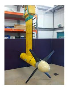
The TTT project involved the testing of medium-scale tidal turbines in three conditions: ideal towing tank tests, steady flow field tests and tidal turbulent flow in Strangford Lough. The 1.5m diameter devices are the first to be tested at the same scale in all three environments. They allow the assessment of the impact of flow condition on performance whilst decoupling the effects of scale.
