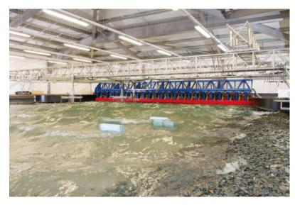
QML has a 18 x 16 m wave basin, with an operating depth up to 0.65 m. The wave tank is equipped with state of the art instrumentation, including a 24-paddle Edinburgh Design Ltd Wave Maker with active wave absorption. The electric paddles can produce regular and random waves with heights up to 0.55 m, wave angle variations from 0° to  $45^{\circ}$  and wave periods from 1 s to 3.5 s.
