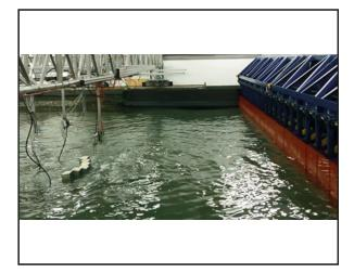
My research is on the assessment of a modular flap-type wave energy converter. The power-capture and foundation loads were evaluated and compared to results associated with a rigid equivalent concept. The assessment was carried out using the QUB Portaferry Wave Tank.
