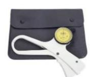
The Holtain Skinfold Calipers instrument has been specifically designed for the accurate measurement of subcutaneous tissue.
