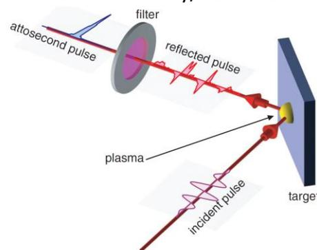
Figure 1 – Sketch of the basic scheme to generate high frequency radiation from a laser interaction with a solid density plasma. Removal of the residual laser energy using appropriate filters can also lead to attosecond scale ( $10^{-18}$ s) pulses - the shortest pulses that it is currently possible to produce. Figure from ref [2]
