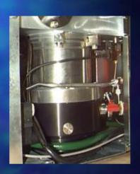
The Turbomolecular pump can pump up to 250L/s. This allows carrier gas flows of up to 5ml/min of helium and can still maintain a vacuum around 2.5 x 10-5 torr.
