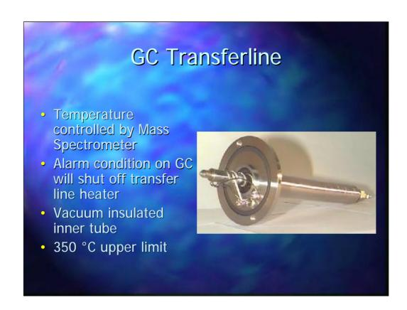
The transfer line connects the AutoSystem GC to TurboMass Gold and guides the column directly to the ion source. The temperature of the transfer line is controlled from the Tune File in the TurboMass Gold software (see Tuning & Mass Calibration section) and is part of the vacuum system of TurboMass Gold.
