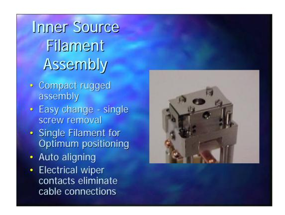
The Filament is part of the inner source and is held in place with a single screw. If a new filament needs to be installed it is a simple operation and the new filament automatically aligns when fitted. The TurboMass gold also has an extended shield over the filament that reduces stray light from the filament and reduces noise
