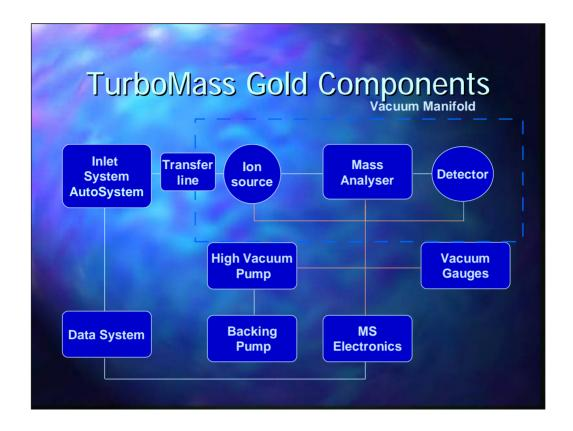
A schematic of the main components in the TurboMass Gold system is shown here.
