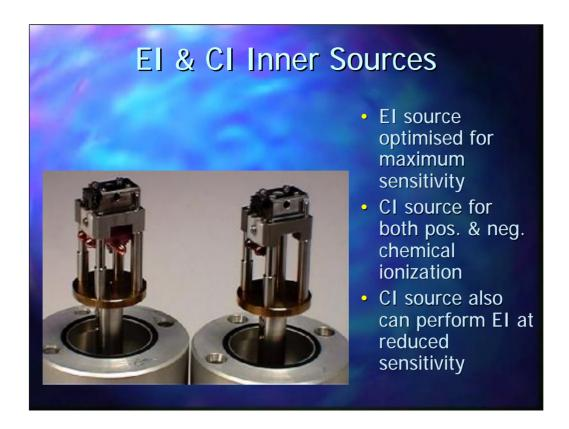
Two inner sources are available. The EI source is optimised for maximum sensitivity for EI+ analysis. A CI source is used for chemical ionisation and may be used in both the CI+ and CI- modes. The ion chamber is designed to maintain the ionisation gas in the ion chamber. It can also be used for EI analysis but with a much reduced sensitivity compared with the EI source.
