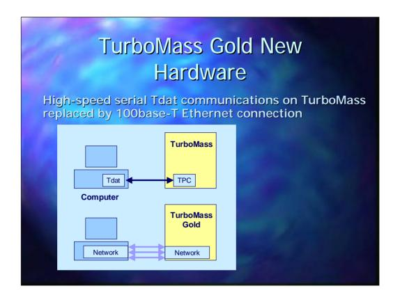
TurboMass Gold incorporates 2 computers, 1 built into the hardware and 1 which is used as the user interface and used to control the GC. The 2 computers are connected by means of an Ethernet connection which gives extremely fast data transfer. This allows mass spectra to be scanned at 6200Daltons/s
