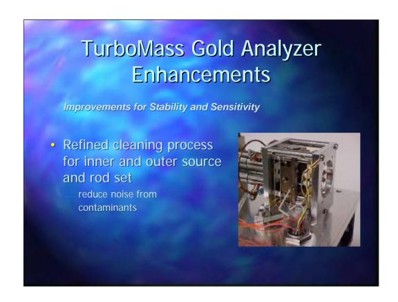
A new cleaning procedure has been introduced with the TurboMass Gold for the inner and outer source during its assembly. This has improved the stability and sensitivity of the system
