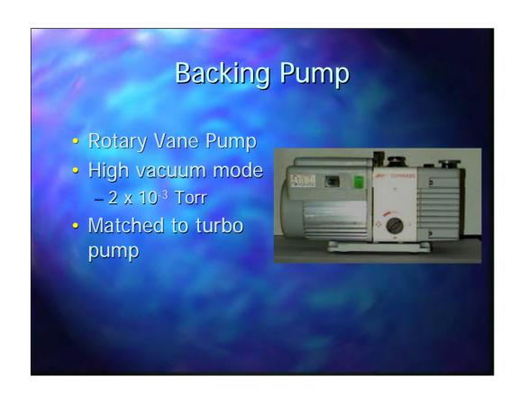
The backing pump is a rotary vane oil pump which is matched to the turbomolecular pump. It is an oil filled pump and the oil must be maintained at the specified levels. The oil should be changed every 6 months.
