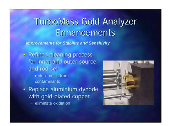
The aluminium dynode that was used in the TurboMass system has been replaced with a gold plated copper dynode to eliminate the possibility of surface oxidation. This, combined with new cleaning procedures for the inner and outer sources and the quadrapole assembly has resulted in a much more stable and higher sensitivity system.
