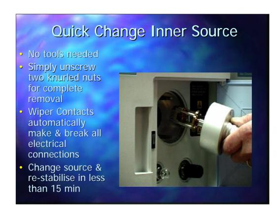
The inner source may be removed and serviced by the user. No tools are required to remove the source, it is simply held in by two knurled nuts. Electrical contacts to between the inner and outer sources are made using wiper contacts which automatically make 7 break when the source is installed and removed.
