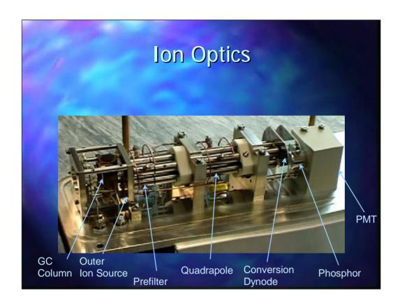
This photograph shows the manifold assembly, including the outer source, prequads, quadrapoles, conversion dynode, phosphor screen and photomultiplier
