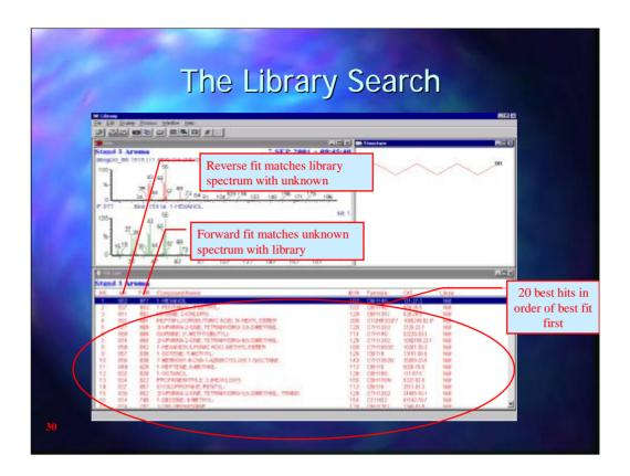
The library search will listed the 20 closest "hits" found in the library to the spectrum from the analysis. The hits are (usually) arranged according to best Reverse Fit match first and Forward Fit match second. The Reverse fit is a measure of how well the ions in the library spectrum match with ions in the sample spectrum whilst the Forward Fit compares ions in the sample spectrum with those in the library spectrum. Both give the match a number out of 1000.
