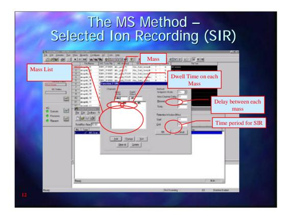
Selected Ion Recording is used for monitoring a single ion or a few selected ions rather than a full a Full Scan. Selected ion recording will give an improved sensitivity over Full Scan and depending on which ion or ions are chosen can be around 50 time more sensitive than Full Scan.
