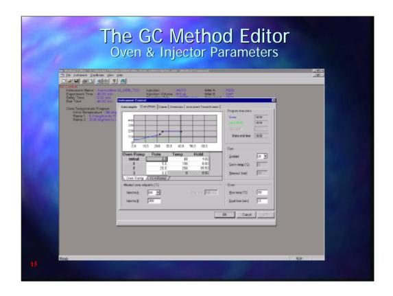
The Oven/Inlets page gives control of the oven and injector temperatures. Note that if a Programmable split/splitless injector is installed the temperature programme is entered by accessing the Injector A and/or the Injector B tabs situated behind the Oven R amp tab. A maximum oven temperature, to protect the column, and an equilibration time, to allow the column to equilibrate with the GC oven temperature after cooldown after a temperature programme are als o entered on this page
