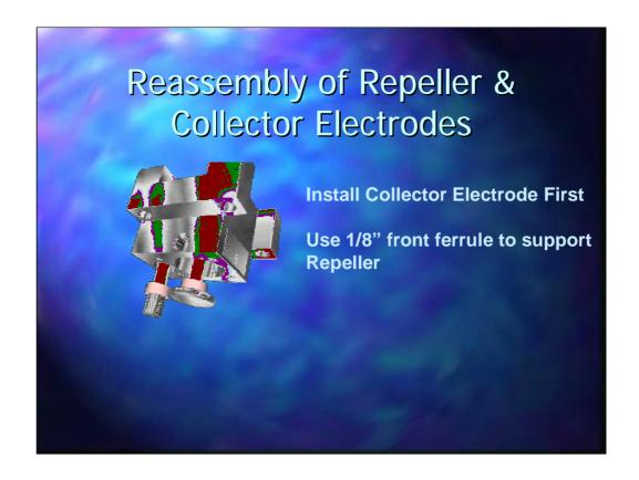
To reassemble the source install the collector electrode first. Slide the long thin ceramic over the electrode followed by the small fat ceramic, ensuring that the first ceramic passes all the way through the second. Holding the electrode in position turn the assembly so that the front of the source is facing downwards and rests on the bench.
