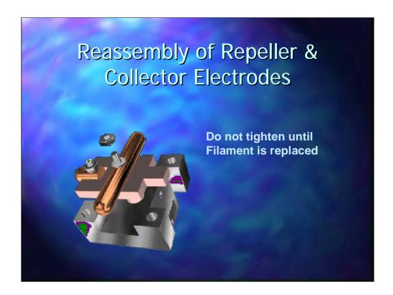
Replace the large ceramic insulator over the repeller ensuring the the collector electrode contact sits between the 2 forks at one end of the ceramic. Place the repeller contact over the repeller with flat surface downwards and a right angles to the collector electrode contact. Fit the washer and then the nut. Loosely tighten the nut but do not fully tighten yet.
