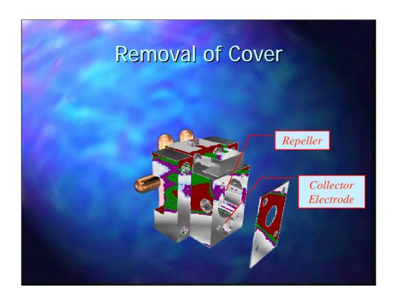
When the cover has been removed the Repeller and the Collector electrodes can be seen
