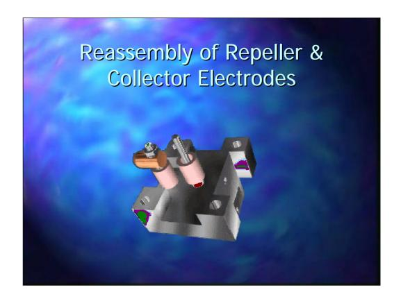
Slide the remaining ceramic insulator over the electrode followed by the contact, the washer and the nut. Tighten the nut loosely at this stage. Repeat the steps for the repeller. However, the repeller sits at the back of the ion chamber and to hold it in the correct position whist the nut is placed on the thread it will be necessary to rest the repeller on a spacer. A Swagelock 1/8 inch brass ferrule acts as a suitable spacer
