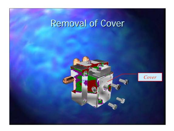
To be able to remove the electrode for cleaning the cover must first be removed from the source by releasing the 4 screws holding it to the source
