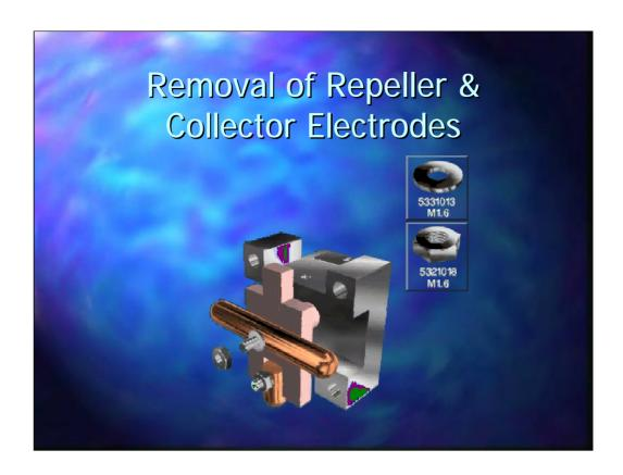
Remove the Repeller by unscrewing the nut holding the repeller contact using the 3.2mm spanner provided in the toolkit and remove the nut and washer
