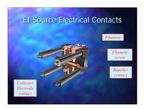
Throughout this series of slides the ion source is shown disconnected from its handle and seal assembly. This has been done for clarity. In practice it is not necessary to separate the 2 parts.
