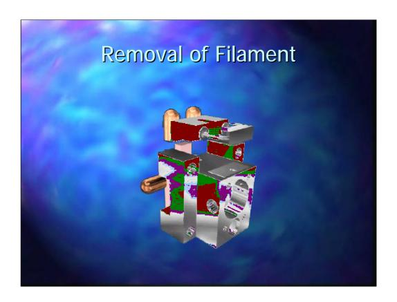
For cleaning the source it is first necessary to remove the filament by removing the screw holding it to the ion source and lifting off the filament.
