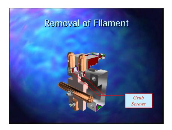
If the filament is broken it will be necessary to remove the contacts from the old filament and put them on the new filament. This is done by slackening the grub screws shown above with the small allen key provided in the toolkit.
