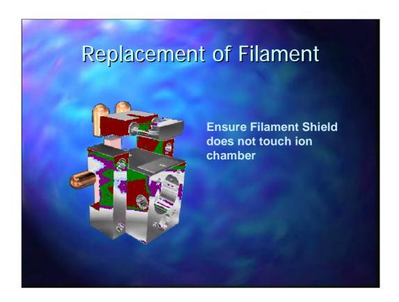
Replace the filament ensuring that as the screw is tightened the filament is pushed so that the screw rests right at the end of the slot in the filament assembly. Check that the cover of the filament is not in contact with the ion source body.
