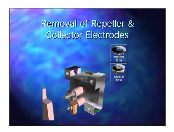
Remove the contact and the large ceramic insulator from the source. Allow the Repeller to fall out of the ion source. There are 3 ceramic insulators around the Repeller, a long thin one, a short fat one and a longer fat one.
