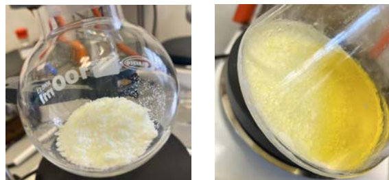
Figure 2 - i) White crystals of trimesitylsilane (first batch). ii) White crystals of trimesitylsilane and yellow liquid which contains impurities (second batch).
