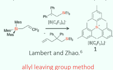
Scheme 4: Synthesis of a 'free' trimesitylsilylium cation.
