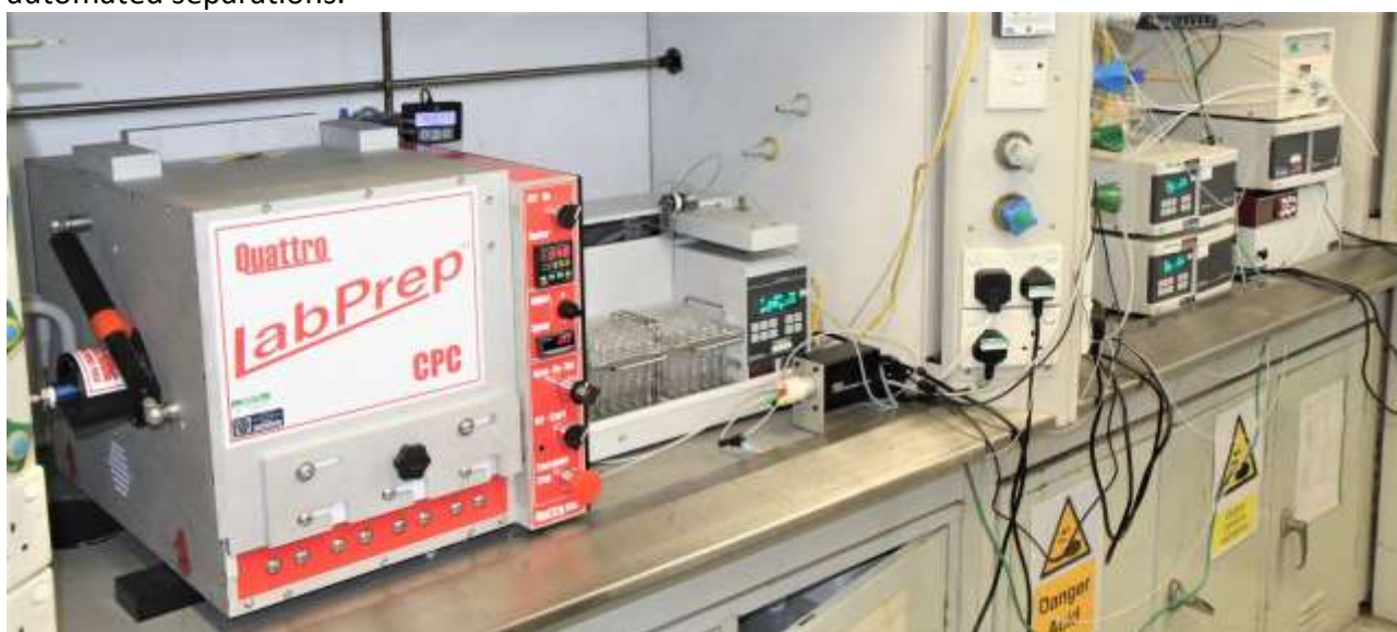
Figure 4 The AECS centrifugal partition chromatography (CPC) machine installed in the QUILL Laboratories.
