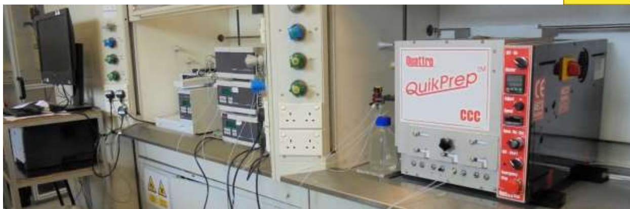
Figure 7 - The IL-Prep™ CCC instrument, pumps, detector, fraction collector, used in the lanthanide separations.
