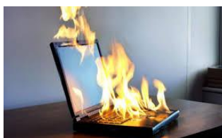
Figure 1-9: Photo of a laptop computer going into fire caused by the overheating of its Li-ion battery.
