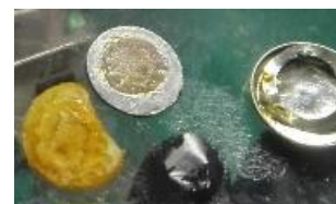
Figure 6-12. Open coin cell showing the [Pyrr 1(201) ][TFSI] decomposition to a yellow colour instead of staying colourless.
