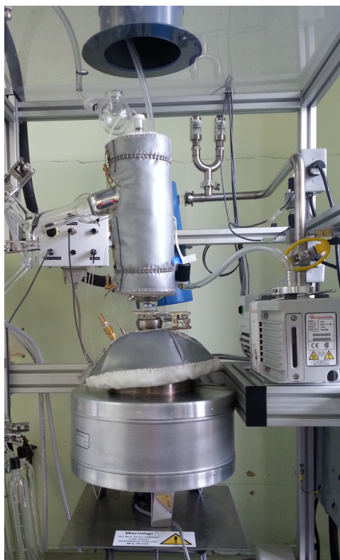
Figure 3.2-3: Distrilab D5236 Crude Oil Distillation System used to fractionate samples
