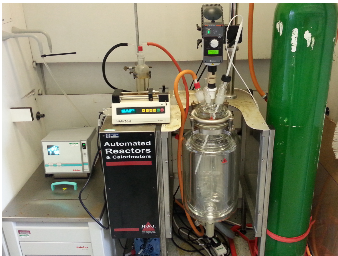
Figure 3.2-2: H.E.L. automated reactor used for large-scale oligomerisations
