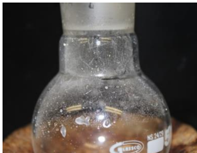
Figure 2.3-1: Ur crystals deposited on the neck of the flask after overnight drying at 80 °C, under reduced pressure
