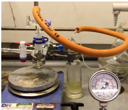
Figure 80. Setup for \text{H}_2 saturation experiments.
