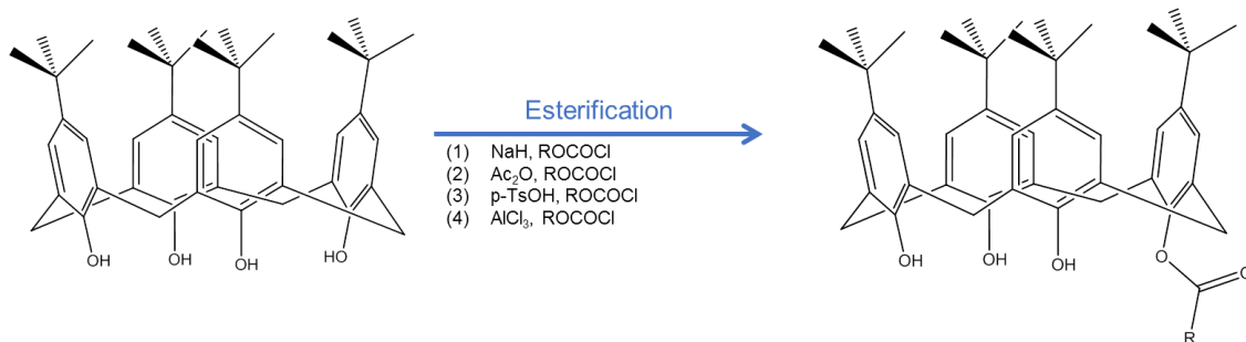
Figure 3-8 —Esterification of p - tert -butylcalix-[4]-arenes with acyl chloride via 4 different methodologies. 220,222
