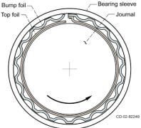
Cross section of foil air bearing
