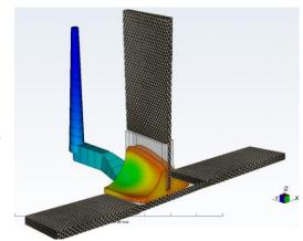
Fig. 1-Flow simulation for a composite overmoulding case
