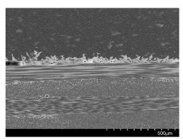
Fig. 2-Interface region in a CFRP overmouled specimen
