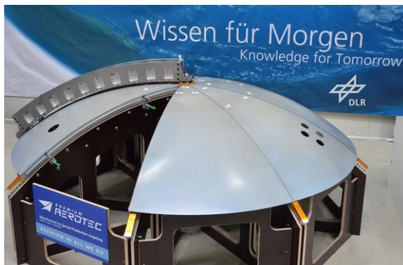
Fig. 1: Thermoplastic rear pressure bulkhead
