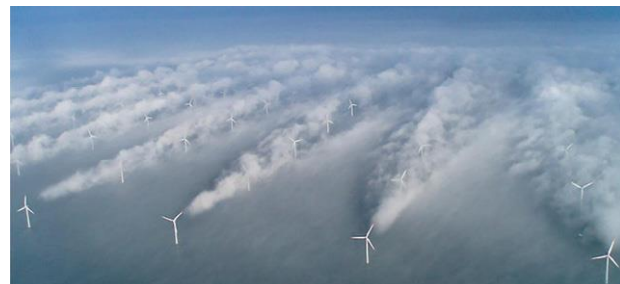
Fig. 5: Wake swirl behind wind turbine
