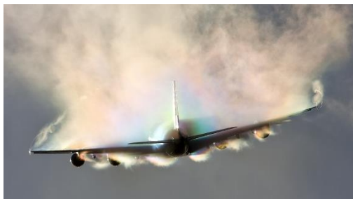
Fig. 4: Vortex shedding behind the airplane
