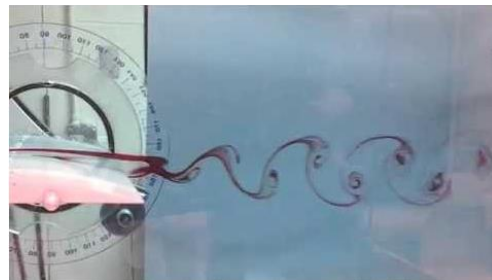
Fig. 3 (b) : Vortex shedding behind an airfoil
