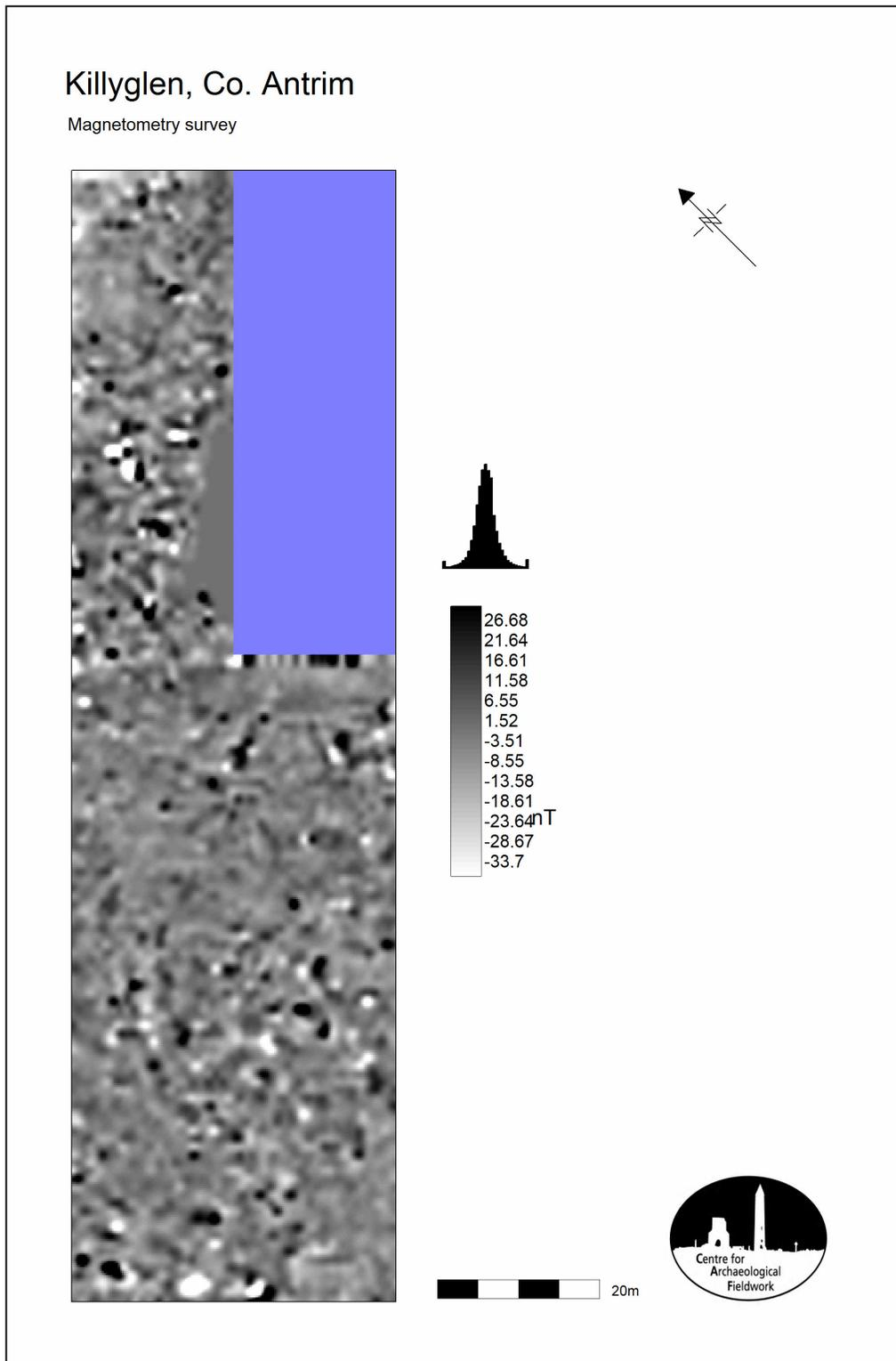
Figure 7. Plot of magnetometry data, showing histogram, colour scale and distance scale.
