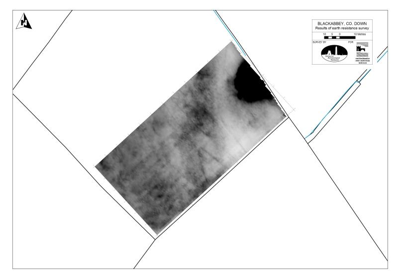
Figure 4. Earth resistance plot overlaid on the base map. Map lines based on Ordnance Survey 1971 1:2500 mapping.
