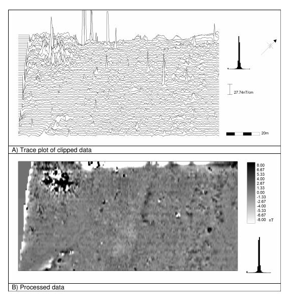
Figure 5. Trace plot and shade plot of the processed magnetometry data from Blackabbey.
