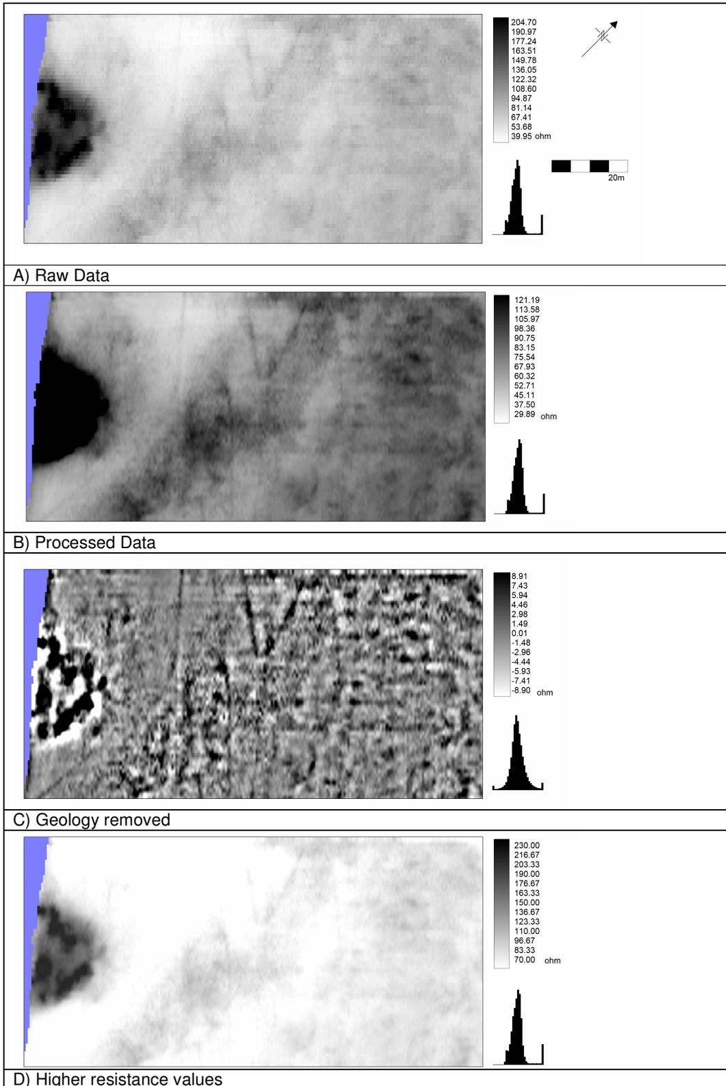
Figure 3. Earth resistance survey data.
