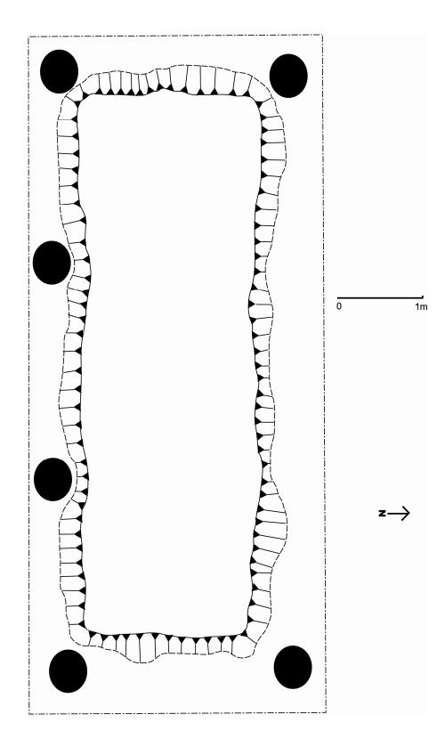
Figure 2: Post excavation plan following excavation of the strip foundations around the piles (shaded black).
