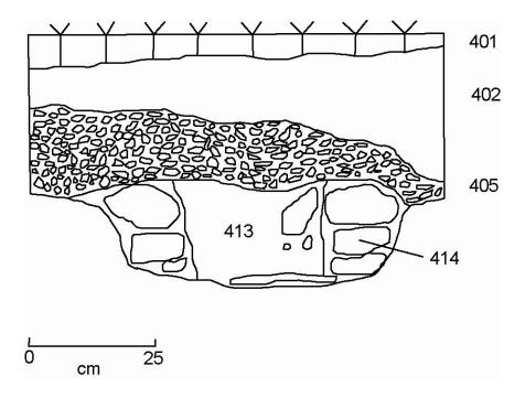
Fig. 8: Section drawing from Trench 4 showing brick lined drainage channel.
