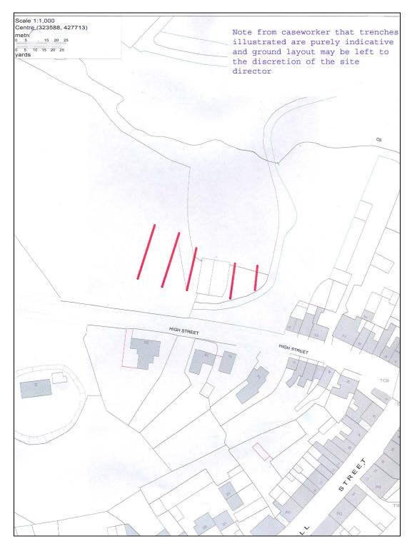
Fig. 3: Map of development site (provided by EHS) showing proposed trench layout. Trenches highlighted in red.
