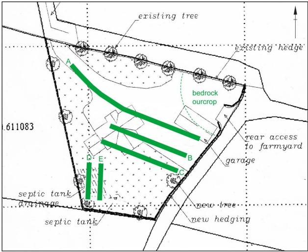
Figure 2: Plan showing application site and approximate location of test trenches. (not to scale)
