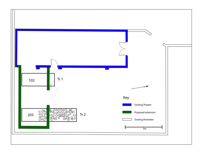
Figure 4: Plan of theatre and proposed extension showing initial Test Trenches.
