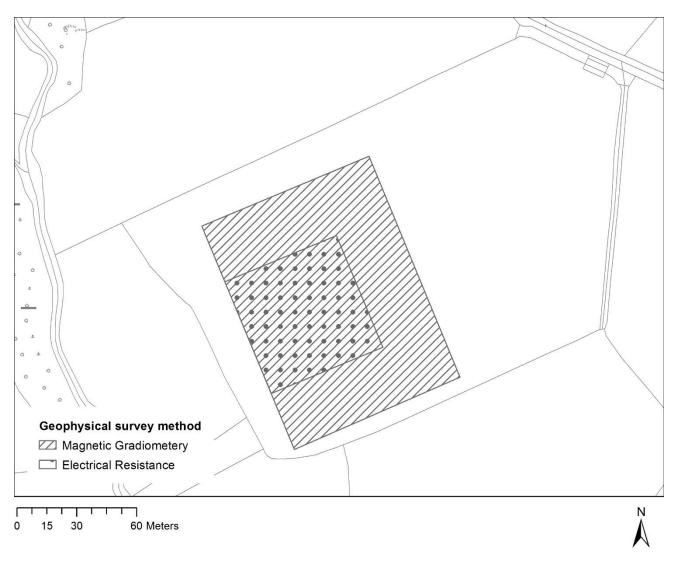
Figure 3 Location of geophysical survey grid and survey methods.
