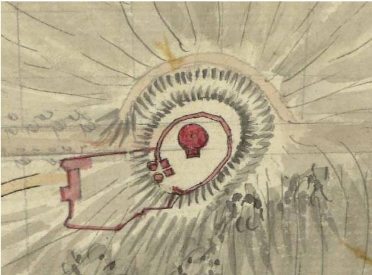
Figure 8: Detail from a Downshire Estate map dated to c.1800 (Public Record Office of Northern Ireland Ref. No. D671.M.5.8.1). The surveyor has depicted the gatehouse between the inner and outer wards as having two drum towers that project beyond the line of the curtain wall. A rectangular extension to the circular great tower is also represented.
