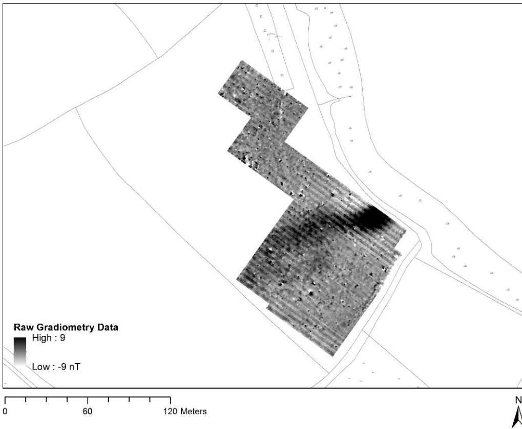
Figure 13 Greyscale plot of Area B1 raw magnetic data clipped to +/- 3 Std Dev.
