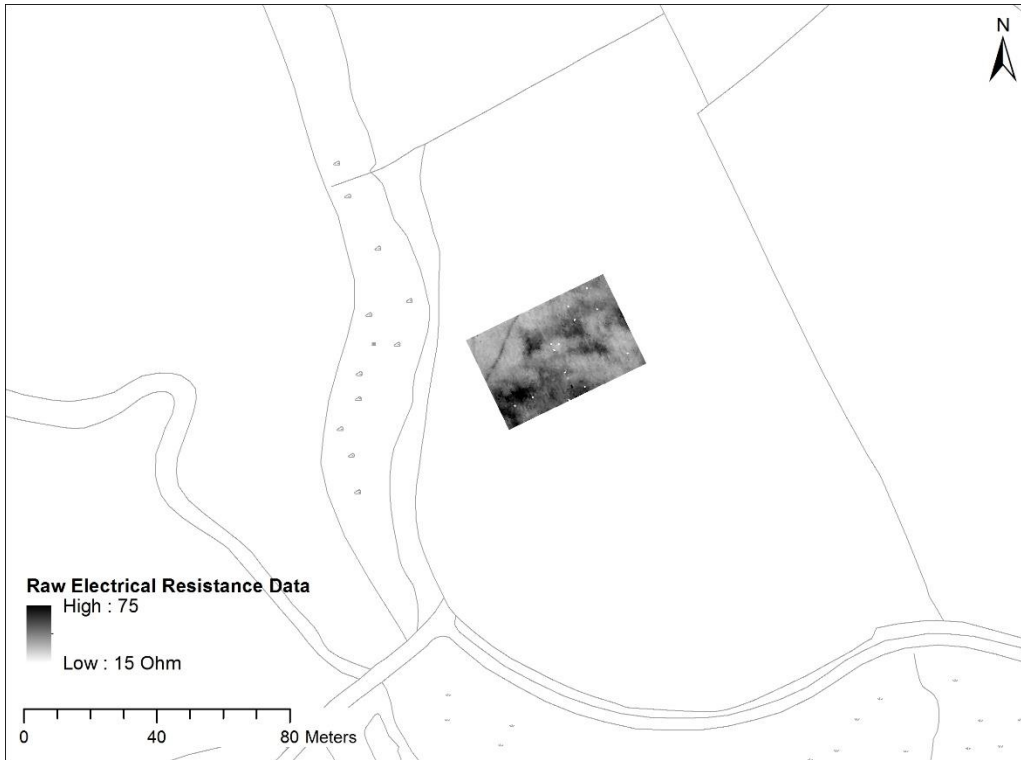
Figure 11 Greyscale plot of Area A raw electrical resistance data Statistics: Mean: 45.26, Std Dev.: 12.36.
