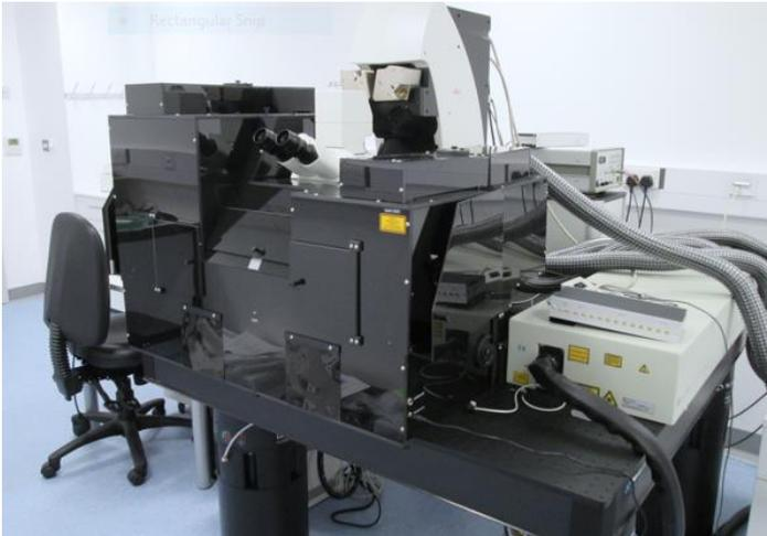
Multiphoton excitation microscopy is a nonlinear event that employs two or more photon with pulsed IR high power laser to excite a fluorophore. Because of the low energy of the IR laser beam it can penetrate deeper within the tissue and generate less scattering, photo-bleaching or photo-destruction.
