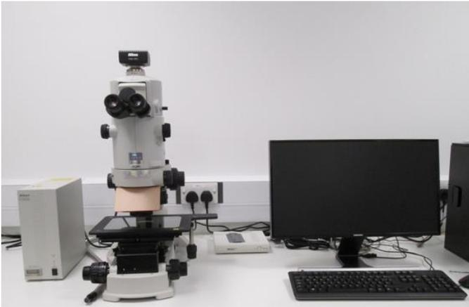
**Epi-fluorescence, diascope Normarski DIC configuration**
