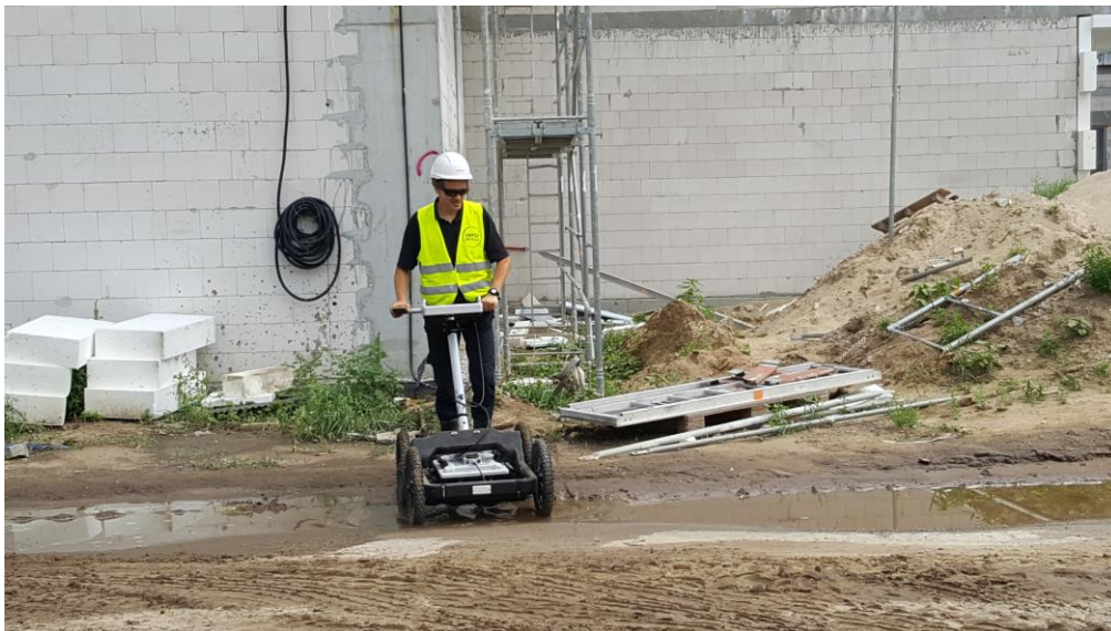
A geophysical search using Ground Penetrating Radar for unexploded ordnance (UXO) in Poland (Photo. Dr Mieszkowski, Department of Geology, University of Warsaw, Poland)
